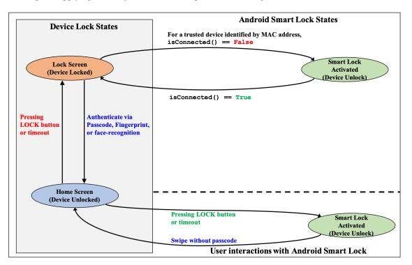
**Figure 2:** The state diagram of the logic that authenticates a device and authorizes access in Android Smart Lock, before applying a patch that counters the attack in 2015. On identifying the connection with trusted device, the logic in Android Smart Lock only check if a connection from registered trusted device (identified by MAC address) is established (or not), and does not check if it is a secure connection or not.
