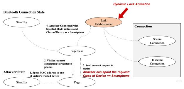
Figure 6: The state diagram of the logic that manages a Bluetooth connection in Windows Dynamic Lock. Windows Dynamic Lock is activated before device establishes any insecure or secure connection to the PC, and thereby, susceptible to our new attack.
