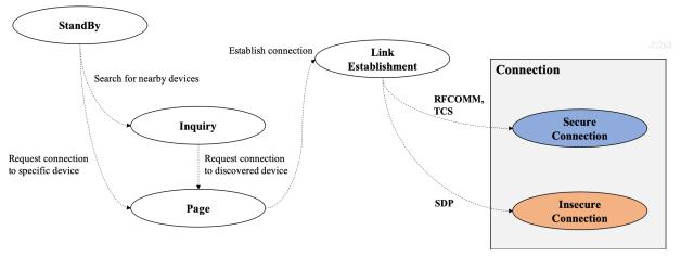
Figure 1: A state diagram of the lifecycle of a Bluetooth connection.
