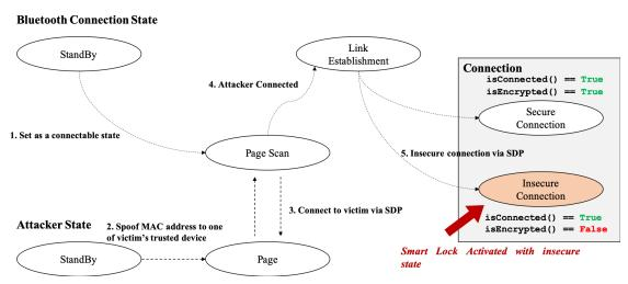
**Figure 3:** The state diagram of the logic that manages a Bluetooth connection in Android Smart Lock. Because Android Smart Lock checks only for the flag isConnected() == True, the attacker may activate Android Smart Lock by establishing an insecure SDP connection.
