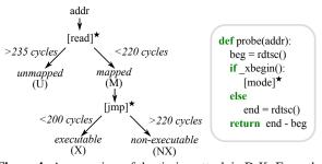
**Figure 4:** An overview of the timing attack in DrK. From the timing differences in calling TSX abort handler for read access (U/M) and execution access (X/NX) inside a transaction, the DrK attack can infer the memory layout of the OS, as well as their permission status (*i.e.*, executable or non-executable). The numbers are collected on a system running Ubuntu 16.04 LTS (kernel 4.4.0), on Intel Core i7-6700K (Skylake) 4.0 GHz processor.
