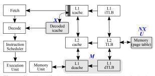
Figure 8: Simplified Intel Skylake architecture including pipeline and cache hierarchy. We omitted L2, last level, and any other page table caches for simplicity. Each M, U, X, and NX indicates the locations where access violation checks are checked according to our measurements. Note that decoded icache, which caches decoded micro-ops, is inside L1 icache [31].
