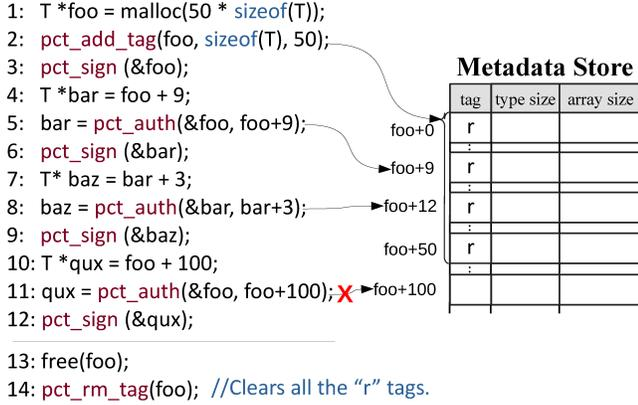
**Figure 5:** Example of PACTIGHT handling array operations.
