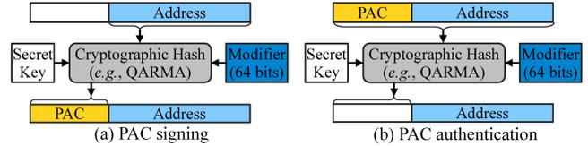
**Figure 1:** PA signs a pointer and generates a pointer authentication code (PAC) based on a address, a secret key, a 64-bit user-provided modifier using PA instructions (*e.g.*, `pacia`). The signed pointer should be authenticated before the access using the same PAC, address, secret key, and modifier using PA instructions (*e.g.*, `autia`).
