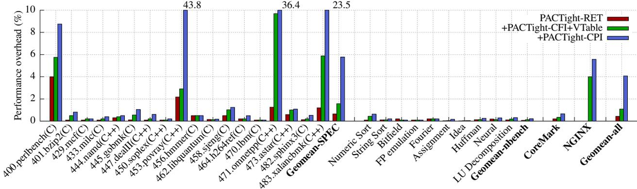
**Figure 8:** The performance overhead of SPEC CPU2006, nbench, and CoreMark relative to an unprotected baseline build. Our three PACTIGHT protections are: 1) return addresses (PACTIGHT-RET), 2) CFI, C++ VTable protection and return addresses (+PACTIGHT-CFI+VTable), and 3) CPI offering full protection for all sensitive pointers (+PACTIGHT-CPI).
