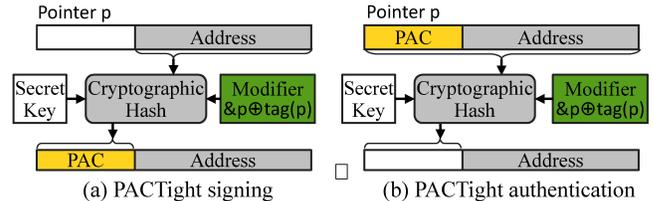
**Figure 4:** Signing and authentication of a pointer variable  $p$  in PACTIGHT. In addition to the unforgeability of  $p$  provided by PA, PACTIGHT uses the address of a pointer ( $\&p$ ) and a random tag associated with a pointee ( $\text{tag}(p)$ ) to provide the non-copyability and non-dangling properties.
