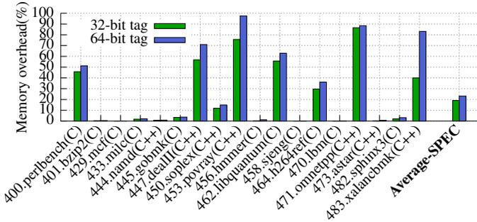
**Figure 9:** The memory overhead of SPEC CPU2006 for PACTIGHT-CPI, PACTIGHT’s highest protection mechanism. PACTIGHT imposes a low overhead of 23.2% and 19.1% on average for 64-bit and 32-bit tags, respectively.
