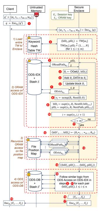
**Fig. 6.** Detailed search protocol.  $\P$  Generate encrypted search query (q).  $\P$  ODS access on ODS-IDX to retrieve file IDs matching with q.  $\P$  Recursive ORAM access on file position map to get the location of matched files.  $\P$  ODS access on ODS-DB to retrieve all matched files and send to the client.
