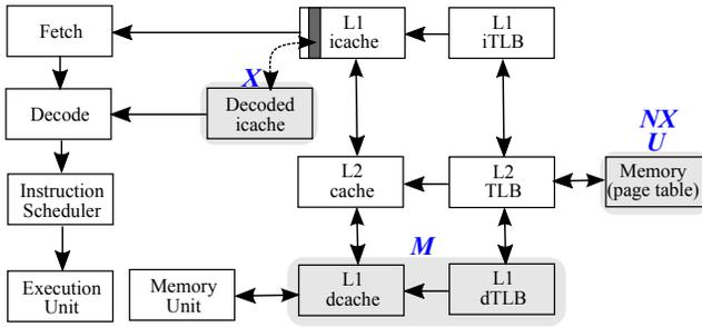
**Figure 8:** Simplified Intel Skylake architecture including pipeline and cache hierarchy. We omitted L2, last level, and any other page table caches for simplicity. Each M, U, X, and NX indicates the locations where page faults are checked according to our measurements. Note that decoded icache, which caches decoded micro-ops, is inside L1 icache [30, 49] and it is a virtually-indexed and virtually tagged (VIVT) cache, which does not require an iTLB access for address translation.
