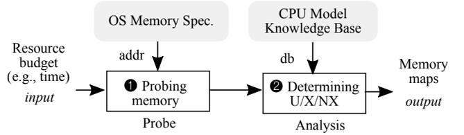
**Figure 5:** Our attack consists of two steps: ① Probing and ② Analysis. ① Given resource budgets provided by users (*e.g.*, time or iteration) and memory specification of the target OS (*e.g.*, maps, types, and page size), we first probe the timing of the TSX aborts in each memory region. ② Then, with the pre-measured knowledge base on the timing characteristics of each CPU model, we determine the memory layout (*e.g.*, mapped regions) and status (*e.g.*, executable regions).
