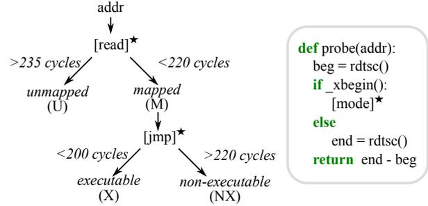
**Figure 4:** An overview of the timing attack in DrK. From the timing differences in calling TSX abort handler for read access (U/M) and execution access (X/NX) inside a transaction, the DrK attack can infer the memory layout of the OS, as well as their permission status (*i.e.*, executable or non-executable). The numbers are collected on a system running Ubuntu 16.04 LTS (kernel 4.4.0), on Intel Core i7-6700K (Skylake) 4.0 GHz processor.
